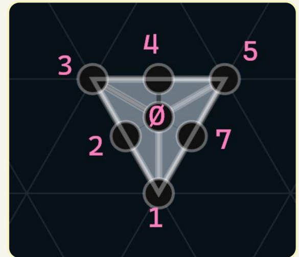
Point-down tile. Socket 0 is the center. Socket 1 is the point of the triangle. The remaining sockets are numbered clockwise.
